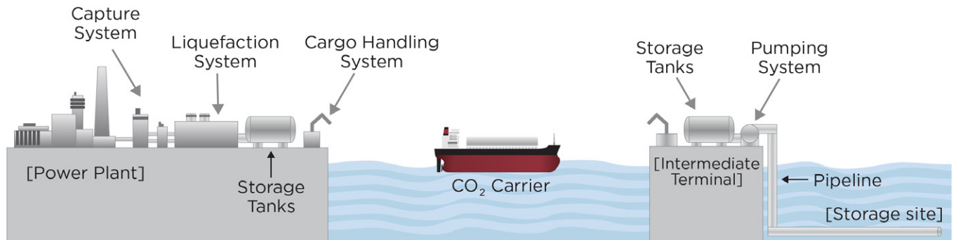
Fig. 2. Carbon dioxide shipping chain
